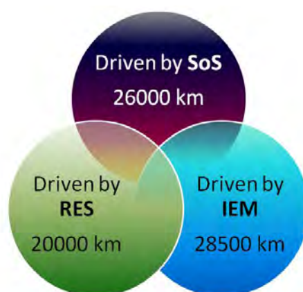
FIG. 2 MAIN DRIVERS FOR INVESTMENT IN NEW OR REFURBISHED POWER LINES (PROJECTS OF EUROPEAN SIGNIFICANCE)
